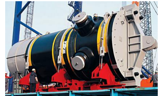
Qinshan Phase II #3 Reactor Vessel
